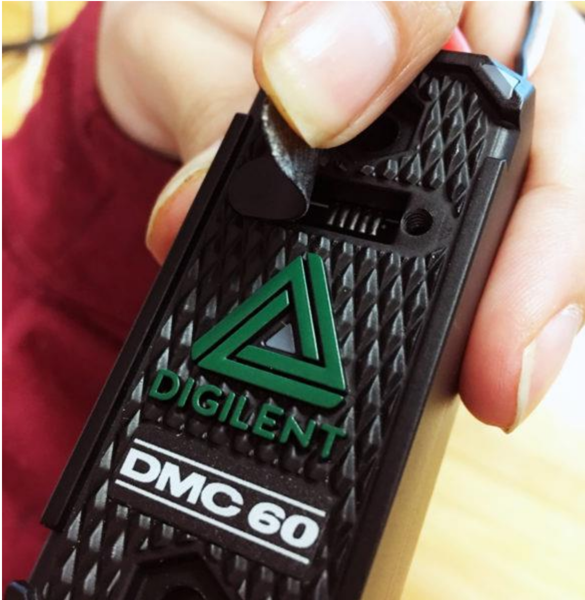
Exposing the programming port for access
