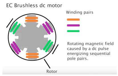
EC motors are controlled by external or onboard electronics that convert the incoming AC power signal to the DC voltage needed by the motor. The electronic circuitry performs the function of the mechanical commutation that switches the direction of the
