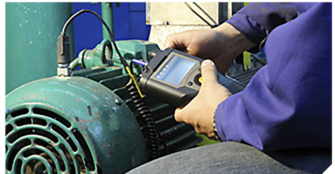
Figure 2. Current approaches to equipment vibration monitoring lack repeatability and reliability.
