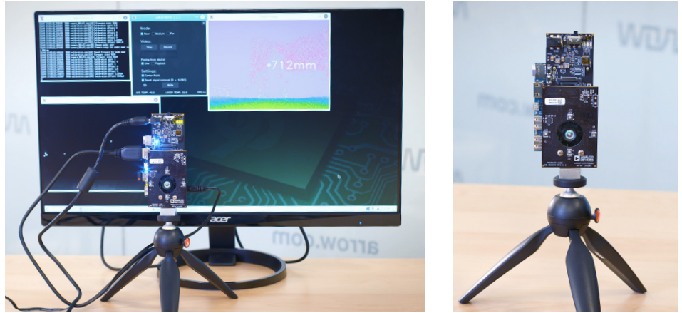
Figure 1: The AD-96TOF1-EBZ covers all product development stages, from evaluation to final application development on an embedded system.
