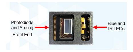
ADPD188BI Smoke Detection Module integrates LEDs, photodiode, and analog front end (AFE) in one small 3.8 x 5.0 x 0.9 mm package
