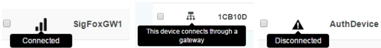
The AuthDevice is not connected since it doesn't utilize MQTT but is only used for authenticate the callbacks.
