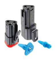
The integrated rear cover on the ML-XT™ housing removes the bend radius from the seal. By seating the rear seal deeper into the connector the rear cover takes this stress, protecting the seal and preventing leak paths.
