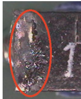
Resistor failure due to the effects of sulfuration. Picture shows silver sulfide (Ag 2 S) needle crystal growth.
