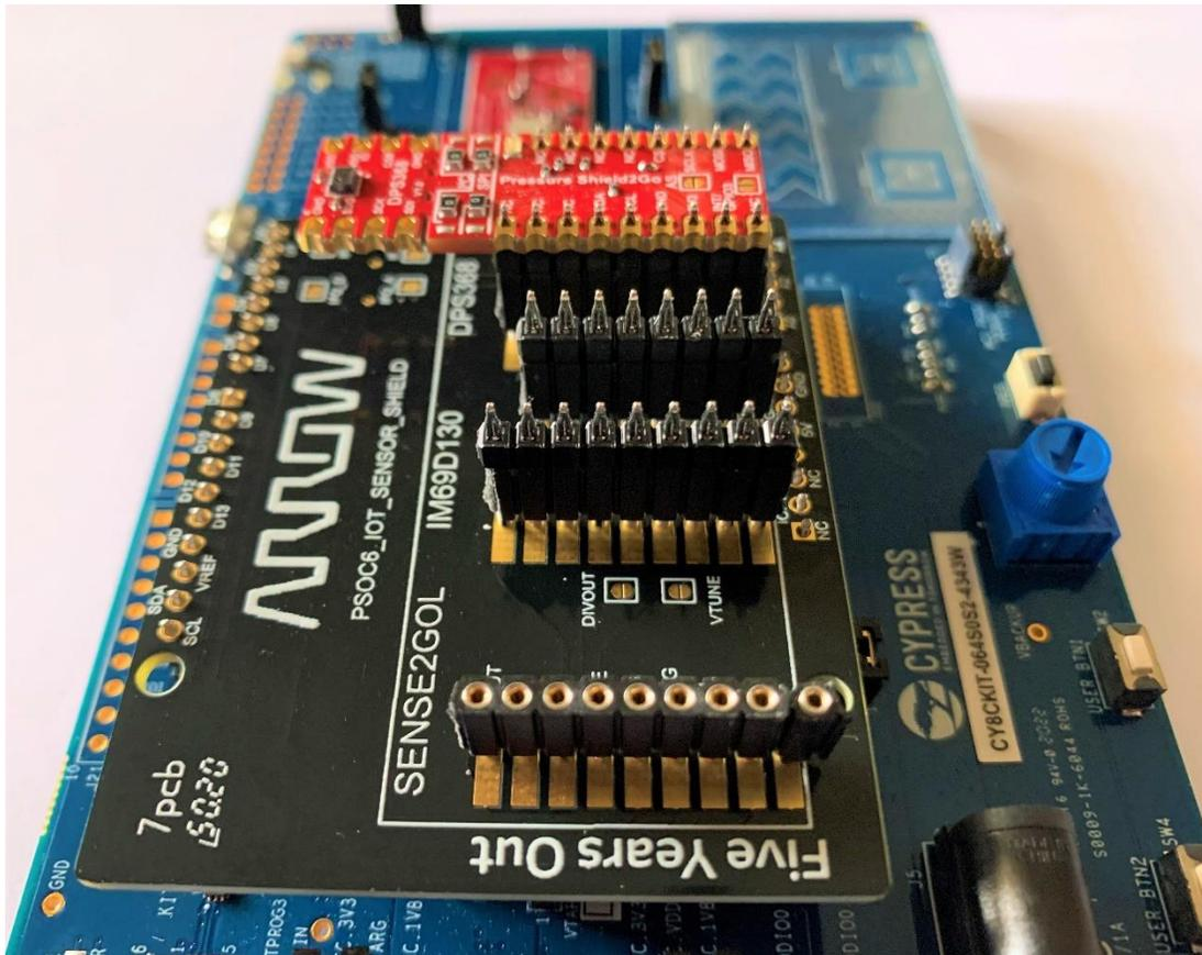
11. Place the IM69D130 Shield2Go board (component side down) on the press fit pins
