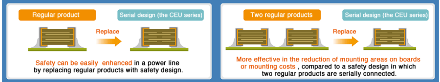
Fig. 12: Image of replacement of regular products with Serial design (the CEU series)
