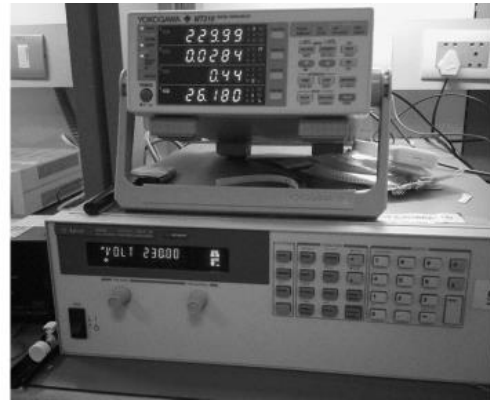
Fig.7 Standby power consumption of LED driver
