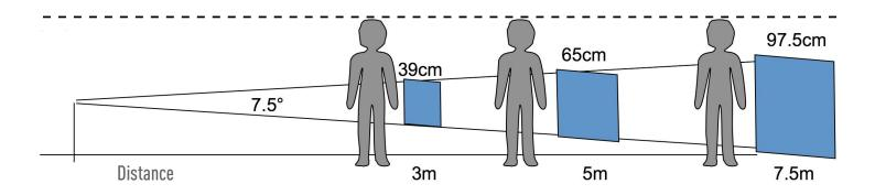
Grid-EYE Sensors can detect human beings across a range of distances. The above diagram shows the field of view for one pixel.
