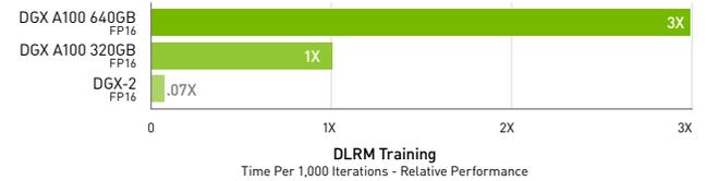
DLRM on HugeCTR framework, precision = FP16 | 1x DGX A100 640GB batch size = 48 | 2x DGX A100 320GB batch size = 32 | 1x DGX-2 (16x V100 32GB) batch size = 32. Speedups normalized to number of GPUs.
