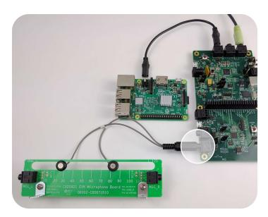
Connect the microphone module to the CX20921 evaluation board (J19)
