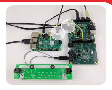
Connect the power supplies for both CX20921 evaluation board, (J10, +5V power supply included) and RPi3 (J1). Switch the power switch (SW3) to turn on the CX20921 evaluation board. LED D6 (5VLED) will turn on when there is power on the board.
