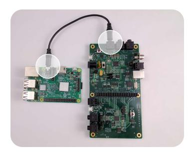
Connect the 3.5mm audio jack on the RPi3 (J7) to LINE IN on the CX20921 evaluation board (J25)
