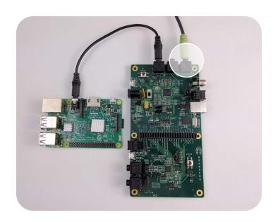
2 | Connect J3 on the CX20921 evaluation board (Line Out port labeled as HP) to a powered speaker
